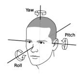
The board incorporates a gyroscope that senses angular velocity in each of three directions. The program integrates the angular velocities to determine angular positions (roll, pitch and yaw). Roll is like tilting your head left or right; pitch is like tilting your head forward and backward; yaw is like turning your head left and right. The program only uses the roll and pitch sensors. Test your code using the C main program. When the program starts (or
