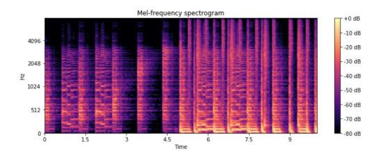
a) Compute the mel spectrogram using a Fast Fourier Transform
