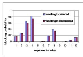
Fig. 8. Blocking probability for the ring topology.
