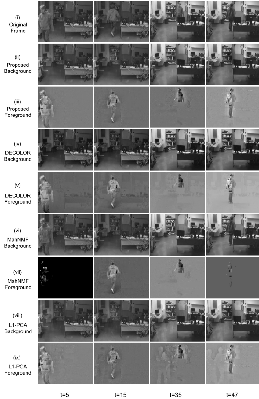
Figure 1: Daniel_light sequence: Original frame [row (i)] of time slot t = 5, 15, 35 , and 47 ; proposed IRW L_1 -PCA reconstructed background and moving objects [rows (ii) and (iii)]; DECOLOR 7 reconstructed background and moving objects [rows (iv) and (v)]; MahNMF 5 reconstructed background and moving objects [rows (vi) and (vii)]; regular L_1 -PCA 11 reconstructed background and moving objects [rows (viii) and (ix)].
