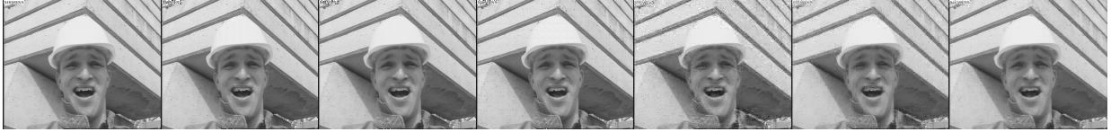
Fig. 2: Foreman for M/N = 0.4 . Left to right: original; FCN+DCT ( T = 10 ), PSNR = 38.44 dB; FCN+DWT ( T = 10 ), PSNR = 38.21 dB; FCN ( T = 10 ), PSNR = 36.73 dB; OMP, PSNR = 26.50 dB; BP, PSNR = 29.15 dB; TV, PSNR = 32.90 dB.
