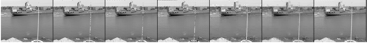
Fig. 3: Container for M/N = 0.2 . Left to right: original; FCN+DCT ( T = 10 ), PSNR = 36.97 dB; FCN+DWT ( T = 10 ), PSNR = 36.90 dB; FCN ( T = 10 ), PSNR = 35.83 dB; OMP, PSNR = 19.47 dB; BP, PSNR = 21.48 dB; TV, PSNR = 24.41 dB.
