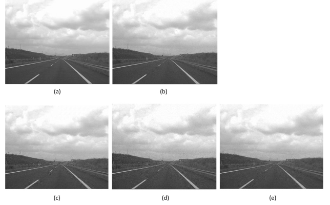
Fig. 5. Different decodings of the 54th frame of Highway . (a) Original frame. (b) Using the proposed order-10 sparsity-aware ME decoder. (c) Using the K-SVD basis decoder [14]. (d) Using the 2-D DWT basis interframe decoder [13]. (e) Using the 2-D DCT basis intraframe decoder [11] ( P = 0.625N ).
