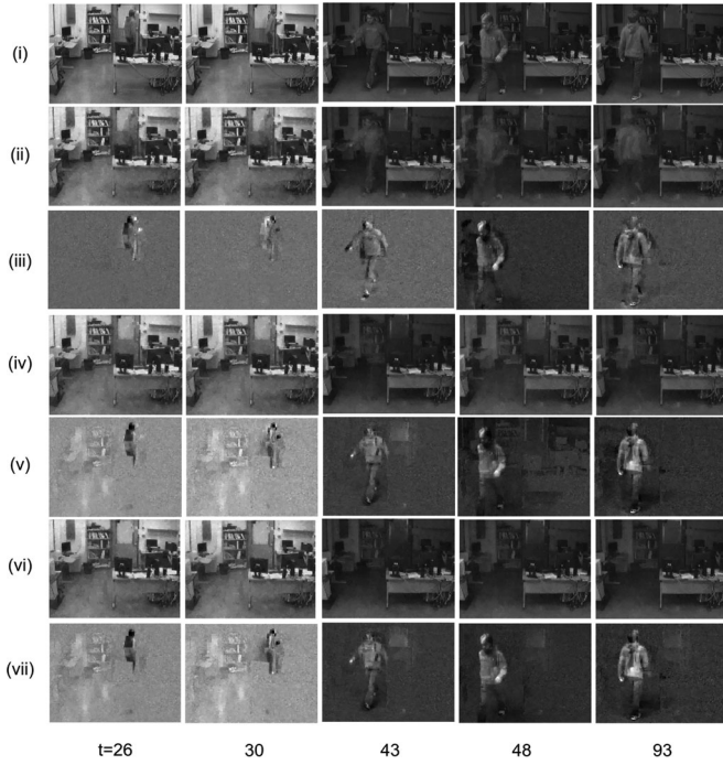
Fig. 8. Daniel_light sequence: original frame [row (i)] of time slot t = 26, 30, 43, 48, and 93 ; non-adaptive CS-L_1 -PCA reconstructed background and moving objects [rows (ii) and (iii)]; adaptive CS-L_1 -PCA reconstructed background and moving objects k = 5 [rows (iv) and (v)]; adaptive CS-L_1 -PCA reconstructed background and moving objects k = 15 [rows (vi) and (vii)].
