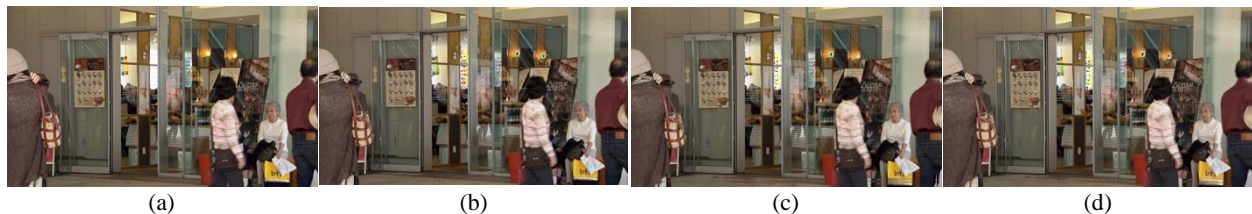
Figure 4. The perceptual quality of the BQ Mall video sequence at the compression ratio 1/12: (a) the original frame; (b) the result of the compression net with SSIM = 0.84; (c) the result of the prediction net with SSIM = 0.82; and (d) the result of the residue network which is our final decoding with SSIM = 0.89.
