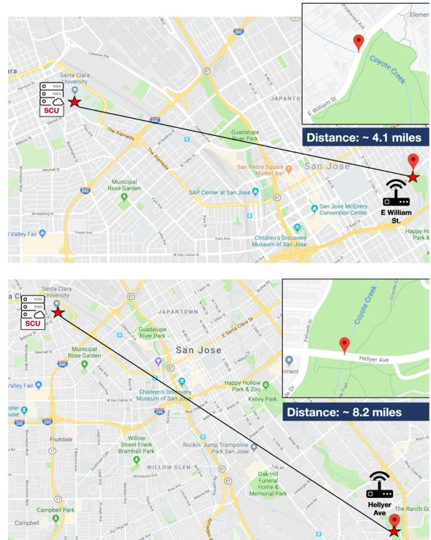
Fig. 5: The Gateway and Nodes use directional antennas to improve connectivity. This figure shows two sample locations where the Nodes were placed and their connectivity with the Gateway were tested.
