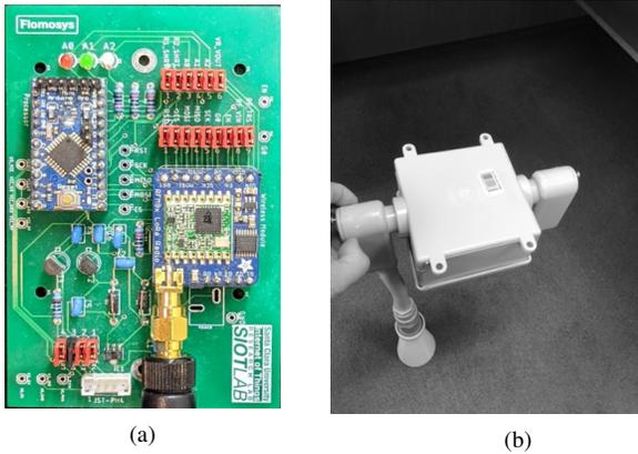
Fig. 2: (a) Node's circuitry, and (b) packaging used for installation on bridges. Low-power circuit design and software improvements were employed to ensure minimum power consumption. The current draw of the circuitry during sleep mode is  $30 \mu\text{A}$ .
