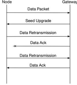
Fig. 6: This diagram illustrates three possible cases for message transmission. The Gateway rejects the first transmission for using an invalid `rand_seqno`, or seed. The Gateway responds with a seed upgrade. The Gateway receives the second transmission, but the ACK message is lost, therefore the Node retransmits the message. Finally, the third transmission is successful, and the Node receives the ACK sent by the Gateway.
