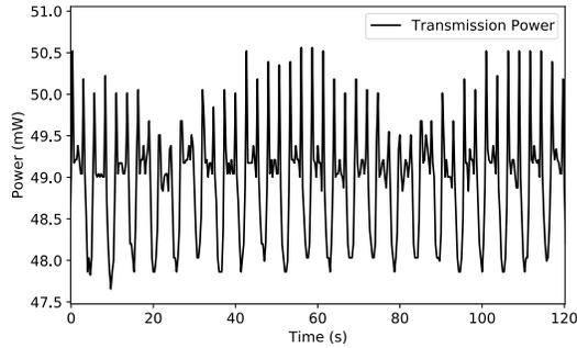
Fig. 3: The power required to transmit LoRa packets over time. Each spike corresponds to a packet transmission.
