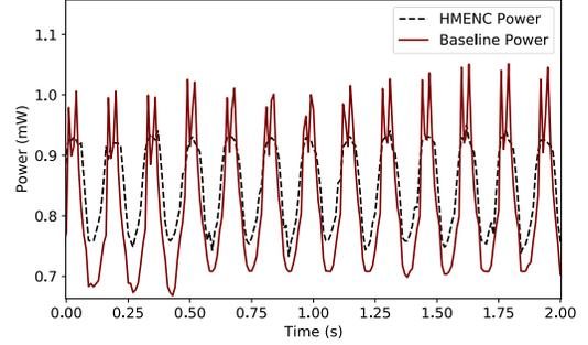
Fig. 8: The power consumption of a full HMENC function performing both memory allocation (on the stack) and encryption. We compare this full function with a baseline function only performing memory allocation.
