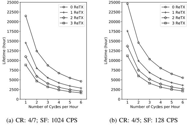
Fig. 9: Theoretical lifetime assuming a 2400 mAh battery with no self-discharge for different average retransmissions, SF, and CR.
