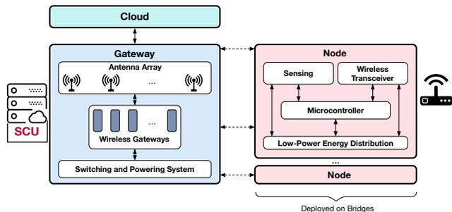
Fig. 1: Flomosys architecture. Each Node measures water level and transmits its data up to several miles away over a secure link to the Gateway. Each Gateway operates on multiple frequencies, performs duplicate packet detection, and forwards the received data to the Cloud. The Cloud provides an administration dashboard for system configuration, as well as data analysis.
