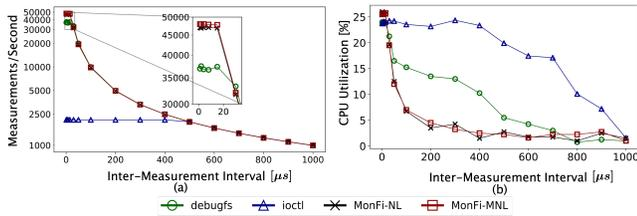
Fig. 2. (a) Measurement collection rate (per second) and (b) average CPU utilization as a function of IMI when using debugfs, ioct1, MonFi-NL, and MonFi-MNL. The monitoring rate of MonFi-MNL is 28% faster than debugfs.
