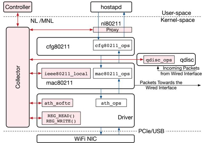
Fig. 1. The architecture of MonFi. The Controller allows use-space programs to specify the type, rate, and method of collecting measurements across the WiFi stack. The Controller collects the requested data from the stack. Various kernel modules have been modified to facilitate collecting monitoring data from them. Note that the hostapd daemon is only used when MonFi runs in an AP.
