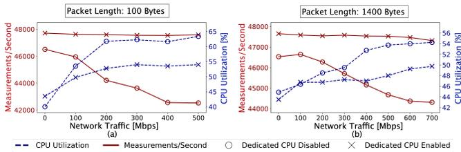
Fig. 4. Measurement collection rate (left y-axis) and CPU utilization (right y-axis) versus packet switching rate for 100-Byte (a) and 1400-Byte (b) packets. These results show that using dedicated cores is necessary to ensure deterministic monitoring rate in the presence of packet switching overhead.
