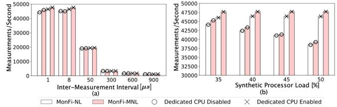
Fig. 3. (a) Measurement collection rate in the presence of a synthetic 30% processor load. (b) Maximum monitoring rate when the synthetic processor load increases from 35% to 50%. Based on these results, using dedicated cores to achieve deterministic monitoring performance is essential.
