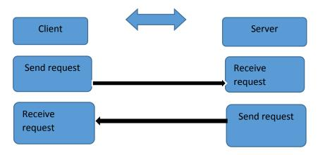
The client sends a request to the server with its IP address and the server gives back a reply with its available port connection and the connection is established.
