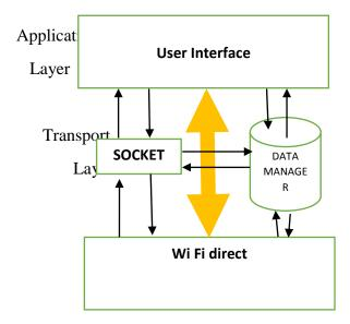
User interface is used to connect to the bottom layers. Connection is established between the two ends. The Data Manager maintains the information about the users. Once the connection is established the two users exchange the profile data and then we determine
