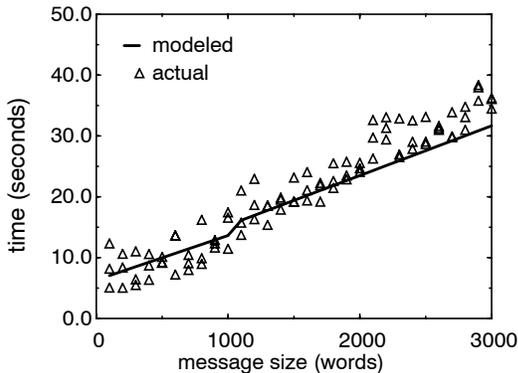
**Figure 6:** Time to send bursts of 1000 equal-sized messages from the Paragon to the Sun in non-dedicated mode, with two processes executing on the Sun, one of which communicates 25% of the time and the other of which communicates 76% of the time.
