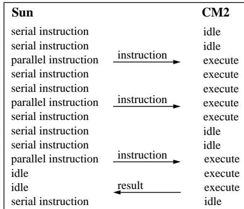
Figure 2: Example of a task executing on the CM2.
