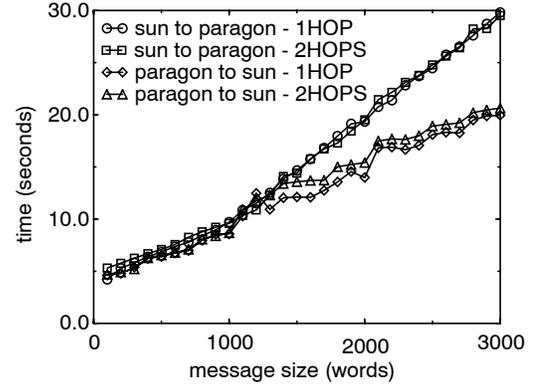
**Figure 4:** Time to send bursts of 1000 equal-sized messages to and from the Paragon in dedicated mode.
