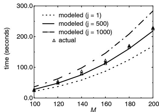
**Figure 8:** Time to execute the SOR algorithm on the Sun in non-dedicated mode with two extra applications executing on the Sun. The contending applications communicate 40% and 76% of the time respectively, and compute the remaining time.
