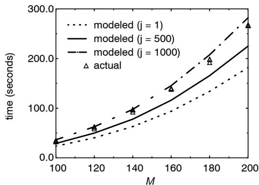
**Figure 7:** Time to execute the SOR algorithm on the Sun, in non-dedicated mode, with two extra applications executing on the Sun. The contending applications communicate 66% and 33% of the time respectively, and compute the remaining time.
