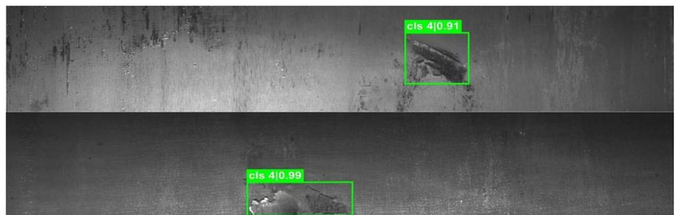
**Fig. 11** The sample detection results on the NEU defect dataset: **a** inclusion, **b** patches, **c** scratches, **d** crazing, **e** pitted surface, and **f** rolled-in scale
