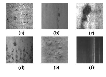
Fig. 8 The NEU defect dataset. a Crazing. b Inclusion. c Patches. d Pitted surface. e Rolled-in scale. f Scratches
