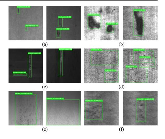
Fig. 12 The sample detection results on the DAGM dataset: a class 1, b class 2, c class 3, d class 4, e class 5, and f class 6
