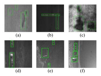
Fig. 1 As a result of defect randomness,  ${\bf a}$  and  ${\bf d}$  show varying scales and  ${\bf b}$  and  ${\bf e}$  show varying directions, while  ${\bf c}$  and  ${\bf f}$  show arbitrary shapes
