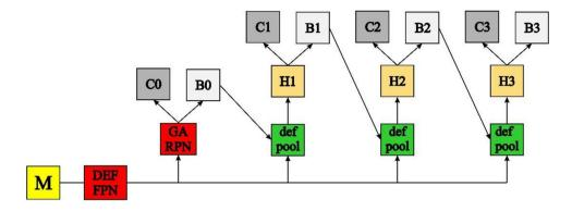
**Fig. 5** The proposed forceful defect detector network, where M is the preprocessing blocks in the training stage and ultimate scaling in the inference stage, DEF-FPN is the backbone feature pyramid network with deformable convolution, GA-RPN is the guided anchoring
